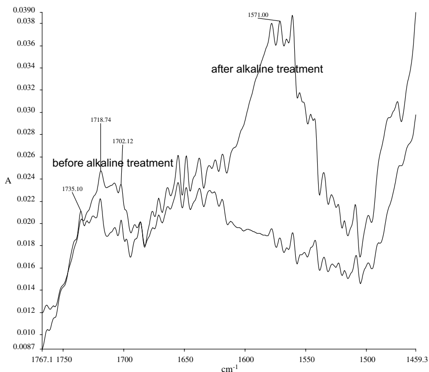
Fig. 4. FT-IR spectra of the finished cotton fabrics (CA was used as catalyst) before and after alkaline treatment.
