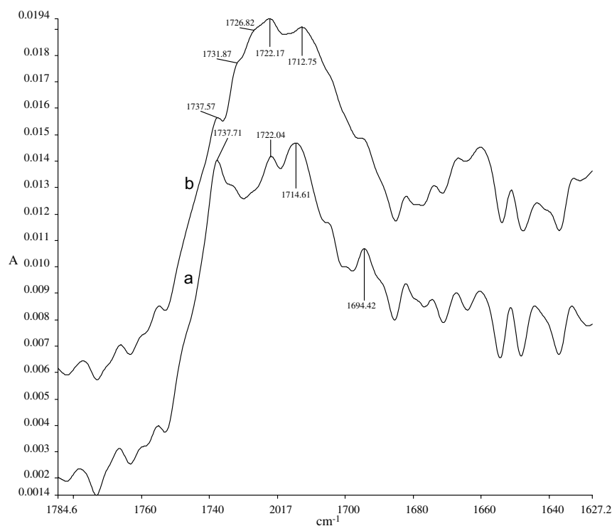
Fig. 5. Differential FT-IR spectra of: (a) cotton impregnated with Rosemary oil and (b) EC/ BTCA/CA finished cotton fabrics (cotton spectrum was subtracted).
